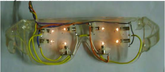
**Fig. 8.** Spectacles with 4 + 4 "lilliput" (LES) 6 volt 60 mA lamp bulbs. These are fitted in plastic "safety glasses"; the right side-piece is clearly visible on the extreme right. The type was selected to have an almost flat-front large area lenses. See text above.
