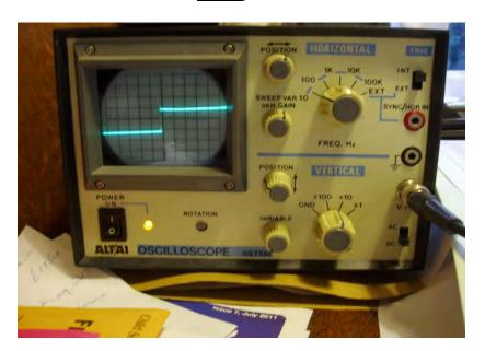
The picture <u>below</u> shows the waveform at either side of the  $0.56~\mu F$  capacitor (on flasher circuit board), showing a sharp rise but a ragged fall. However, the final result across the lamp terminals is all that is necessary (the picture <u>above</u>).
