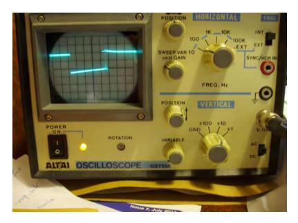
Above picture shows sharp rise & fall of square wave edges, measured at the lamp bulb terminals. The scope happened to be set to "AC input", but the picture <u>below</u> was set to "DC input" and shows a squarer square wave. The vertical DC voltage difference between the two lines <u>below</u>, is 1.5 volts:
